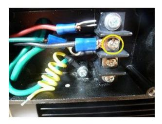
Step 5 Connect the red (hot) line to L2 on the terminal board. If L2 is not visible on the terminal board, see picture for location.
