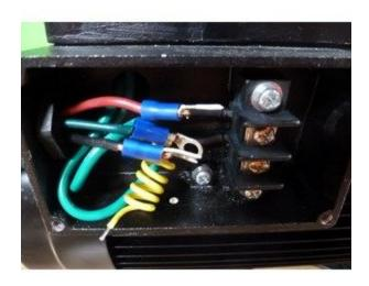
Step 4 Connect the black (hot) line to L1 on the terminal board. If L1 is not visible on the terminal board, see picture for location.
