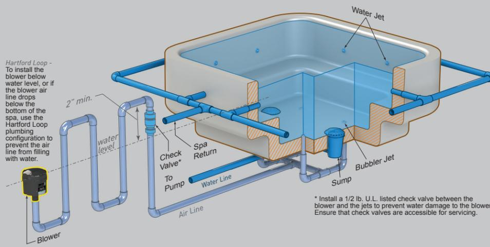
\* Install a 1/2 lb. U.L. listed check valve between the blower and the jets to prevent water damage to the blower. Ensure that check valves are accessible for servicing.
