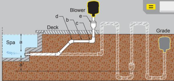
**NOTE:** Include a' for installations with a check valve below the air outlet only. See "Below Grade Installation" on facing page for details. For above grade installations enter 0 for a'.
