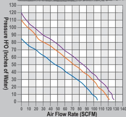
Locate the total back pressure, calculated above and draw a horizontal line. Locate the total airflow from previous step and draw a vertical line. These lines will intersect on the performance curve of the minimum HP blower required for your application.
