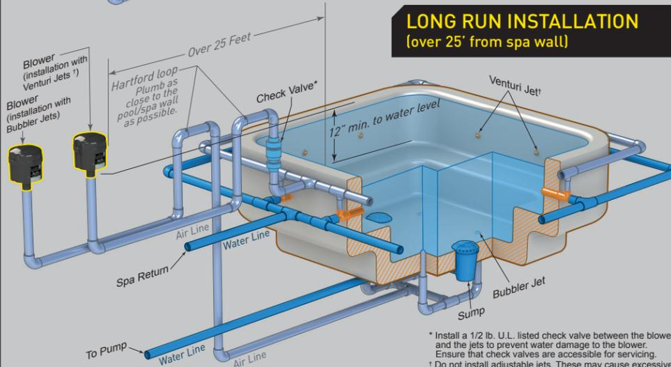
\* Install a 1/2 lb. U.L. listed check valve between the blower and the jets to prevent water damage to the blower. Ensure that check valves are accessible for servicing.
