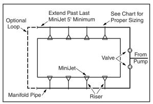
3. When the MiniJets are lined up to project water streams of equal distance, cut the risers to equal lengths. When the MiniJets are not set in lines parallel to the pool edge, valve each MiniJet separately.
