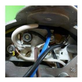
Step 10 Connect the green (ground) line to the copper screw with initials GRD molded next to it.
