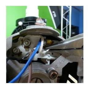
Step 4 Move the white motor line from terminal 4 to 1.
