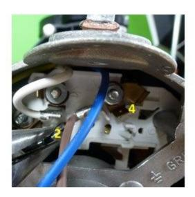
Step 6 Move the black thermal protector line from terminal 2 to terminal 4.
