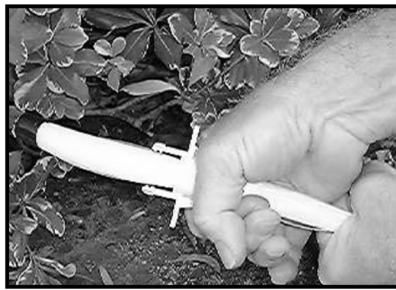
5. Pull on ferrule to check tightness.
