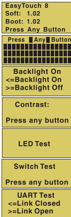
Press the **Right** button to display the current software and bootloader revision levels for the EasyTouch indoor control panel.
