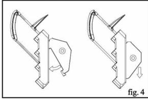
4. Slide the fence into the step and push it towards the foot of the step (Fig. 4). **CAUTION: The safety fence is not supposed to touch the**
