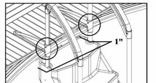
5. Lower the step into the water. Move it to its permanent location and level it horizontally.
