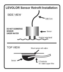
The Sensor is half-moon or 1" slip style with 50 ft. - 200 ft. of wire at the top and two stainless steel contacts at the bottom. The half-moon Sensor can be mounted with a suitable adhesive in the skimmer throat behind the whir door arc.
