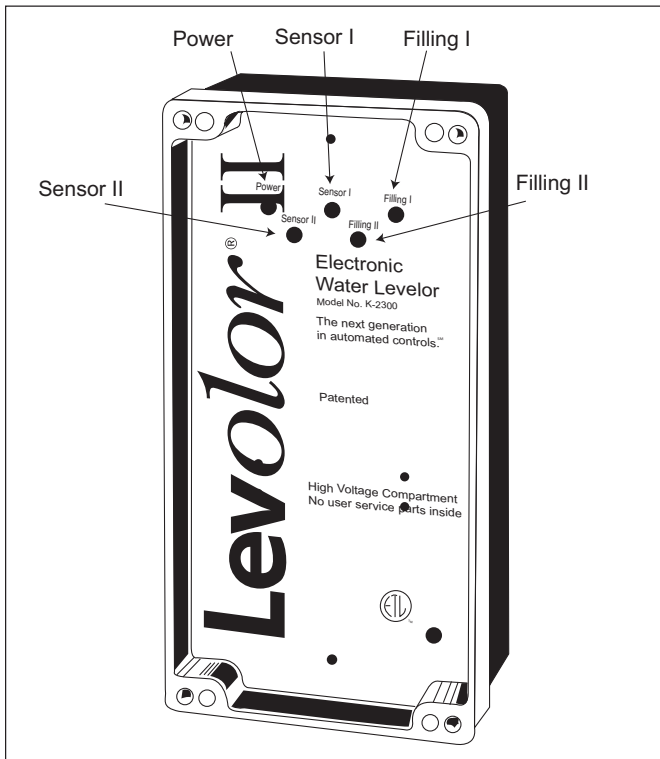
Figure 24. K-2300 Controller Lights
