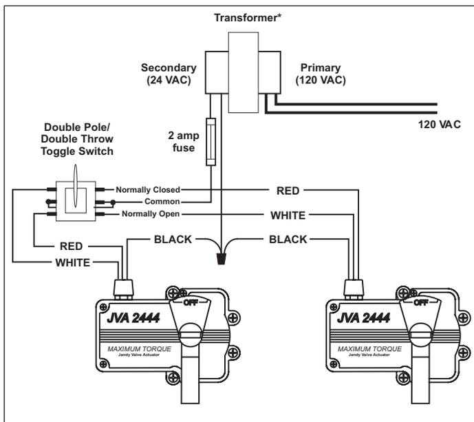
\* Transformer must be sized for the number of JVA's. Each JVA requires .75 amp. at 24 VAC.
