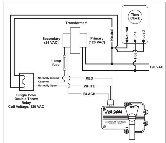
\* Transformer must be sized for the number of JVA's. Each JVA requires .75 amp. at 24 VAC.
