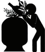
Never attempt to adjust or remove the lid when the pump is running or there is pressure in the system. This can cause product failure or also cause the filter lid to be blown off which can result in death, serious personal injury, or property damage.
