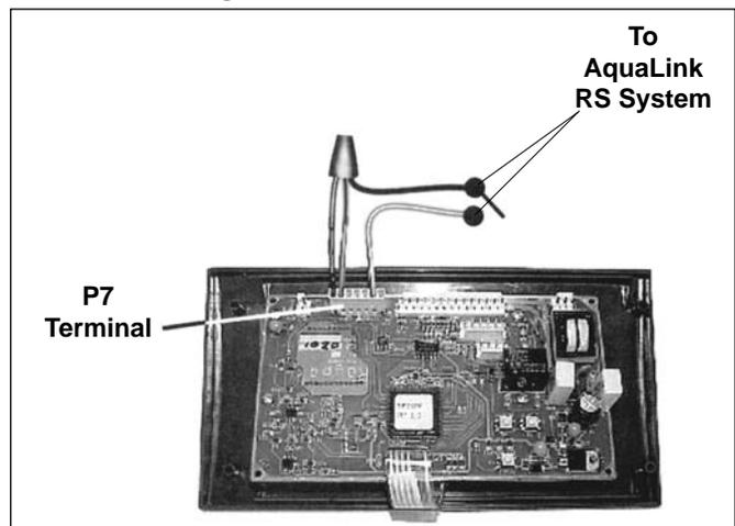
Figure 15. Raypak Heater Wiring with AquaLink RS
