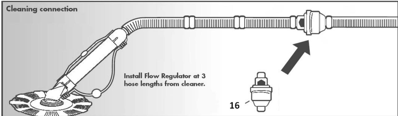
9. Turn your pump on and observe the cleaner's movements around your pool. You may need to install the Flow Diverter(s) to redirect return water to permit your cleaner to cover your entire pool area.
