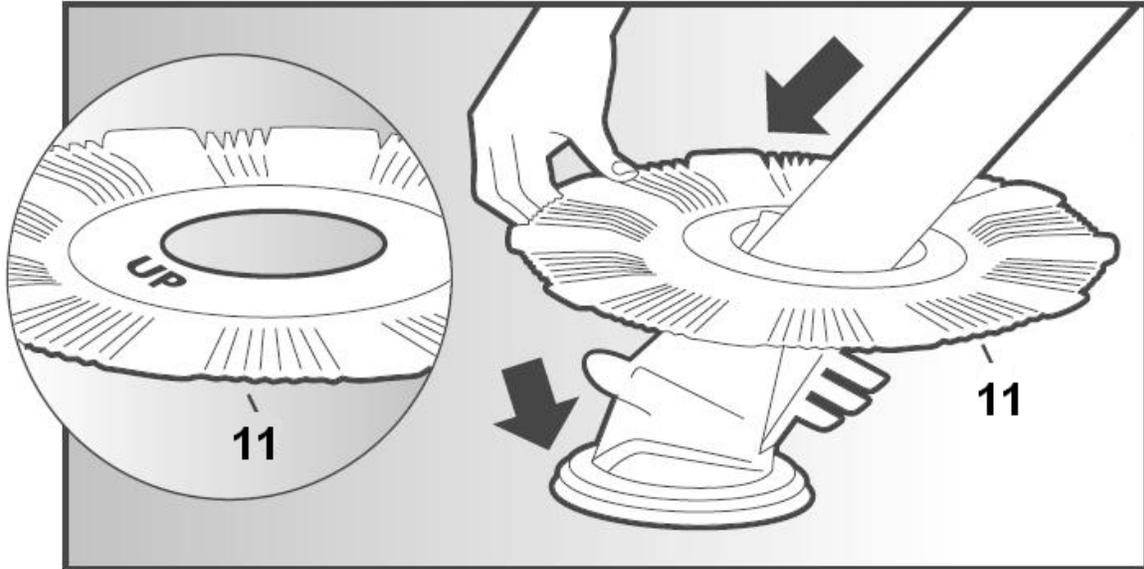
2. Install the Handle by flexing and inserting each end into the slots on top of the cleaner. Install the Deflector in the same manner under the cleaner insuring the weight is towards the bottom.
