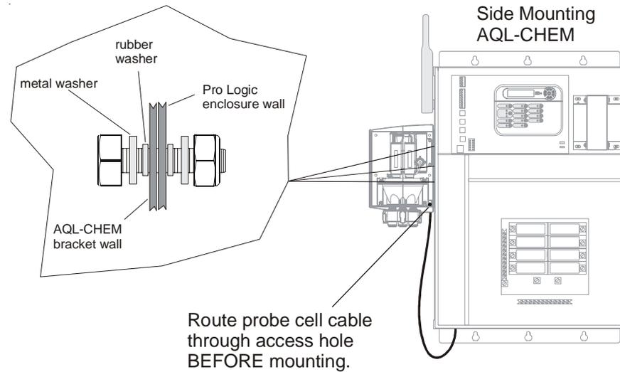
**Remote surface mounting the AQL-CEM:** The Probe Cell can be mounted up to 15' away from the Pro Logic (limited by length of cable). Use the four mounting holes on the back of the bracket when surfacing mounting. Common wood screws can be used for most applications.
