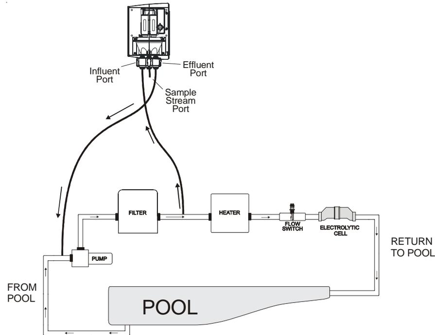
Drill and tap a 1/4" NPT hole using a 7/16" drill bit on the return side of the pool plumbing at a location just downstream of the filter, but upstream from the AQL-CL Electrolytic Cell. Use caution not to tap tapered threads too deeply. Using teflon plumber's tape, install a tubing connector into the hole. Run flex tubing from the tubing connector to the influent Probe Cell port. Push flex tubing in fully to seat.
