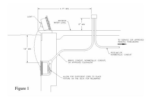
Install fixture in a vertical pool or spa wall – not in floor. Failure to install the fixture properly could result in personal injury and/or property damage.
