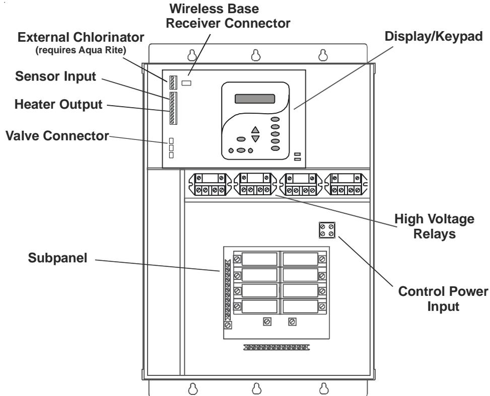
The ECOMMANT 4 Control Center requires both high and low voltage connections. Low voltage connections will be made to actuators, sensors, remote keypad, etc. High voltage connections will be made to pumps, lights, etc., as well as providing direct input power to the Control Center. Always:
