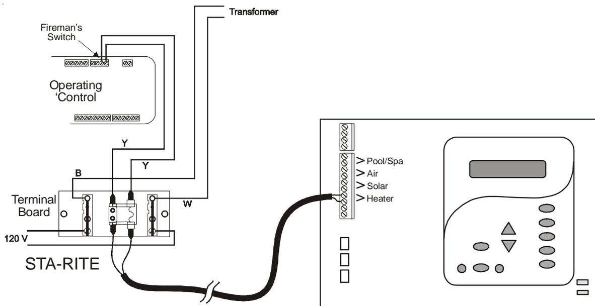
**Hayward Variable Speed Filter Pump:** Refer to the diagram below for proper low voltage communication wiring between the ECOMMANT 4 and the Hayward Tristar Variable Speed Control (VSC).
