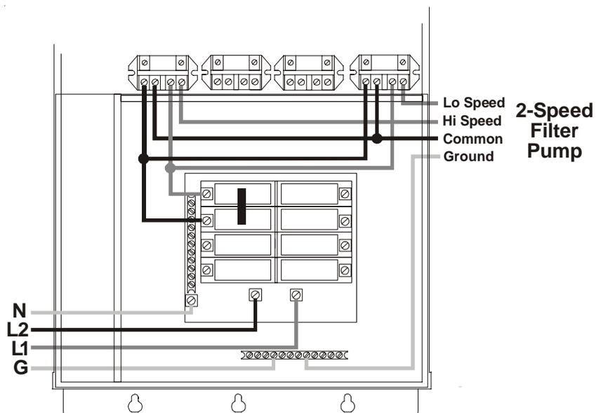
**Lights:** A ground fault circuit breaker must be used to supply power for high voltage pool/spa lighting. Low voltage lights will require an external transformer. For lighting systems that have both a light source and color wheel, connect the light source to the “Lights” relay and then connect the color wheel to one of the AUX outputs.
