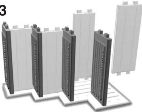
Insert a riser between each of the steps so that the ends of the risers align in the riser recesses on the same panel.
