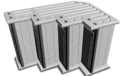
Position the second side panel over the steps and risers and press the panel down so that each step and riser are fully seated into the second side panel. It may be necessary to tap the side panel, using a mallet or a hammer and block of wood, to fully seat it.
