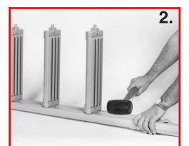
Tap the tread downward so that it seats fully into the bottom of the keyhole slot. Repeat above procedures using three more treads. Do not attach the bottom tread at this time.
