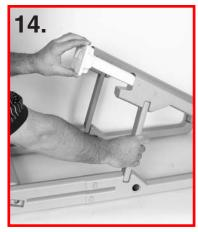
Slide the assembled tube/block assembly up into the open end of the handrail return as shown.
