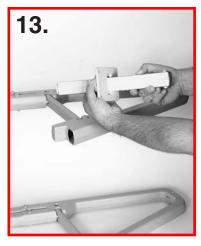
Coat the adjustable tubes with a small amount of liquid soap or lubricant and slide the tube up through the mounting block as shown.
