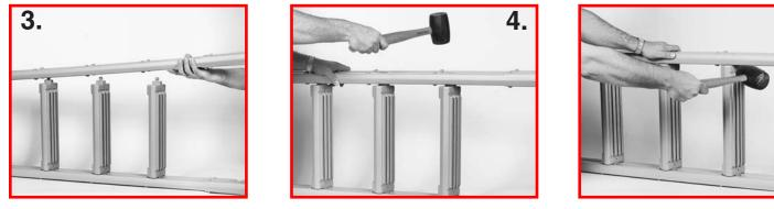
Attach one of the ladder legs to the opposite ends of the four treads making sure that the curved upper ends are both facing in the same direction. Tap the treads into place making sure that they are fully seated into the keyhole slots.
