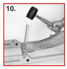
Lay the ladder section down as shown and tap the two handrail connectors into the slots with the warning labels facing up.
