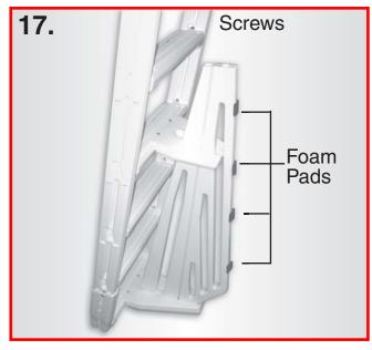
Place the Base and Brace into position, centered, on the bottom and fourth treads of the ladder. Install the four (4)  $\#10 \times 1-1/4"$  screws (included in hardware pack) on a slight angle, first in the Upper brace, then in the Lower Base. Install the self-adhering foam strips to the Large Barrier Section as shown in diagram.
