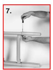
Using two (2) #10 x 2" bolts and two (2) acorn nuts, fasten the extension boots to the ladder legs.
