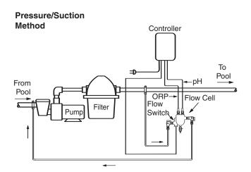
3. Plumb from before the filter to after the heater, using an inline filter to minimize the possibility of debris coming into contact with the sensors.
