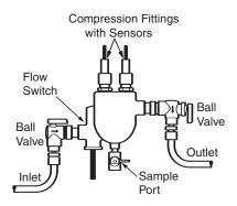
There are three suggested methods to install the flow cell.
