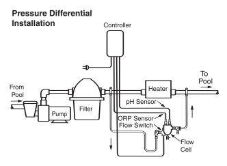
Plumb from after the filter to before the pump. This ensures excellent flow but the flow must be adjusted so the sensors are not subjected to a suction environment. Open the sample port (see Flow Cell Assembly drawing) to verify that water is flowing freely from it.
