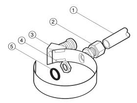
**If using a pipe tap**, drill a 7/16" hole and tap a 1/4" NPT hole. Apply RTV silicone, teflon stick or teflon paste to the threads on the Jaco fitting and screw securely into the pipe. Test for leaks.
