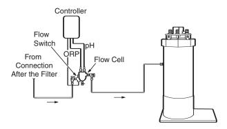
Be aware that solar systems and other factors can alter pressure differentials in a system, adversely impacting flow through the flow cell. The flow cell comes fully assembled. It is setup to use the 3/8" tubing provided; however, other sized tubing or 1/2" hard plumbing can be used. To use an alternative tubing, remove the 90° on/off valves and plumb according to the application.
