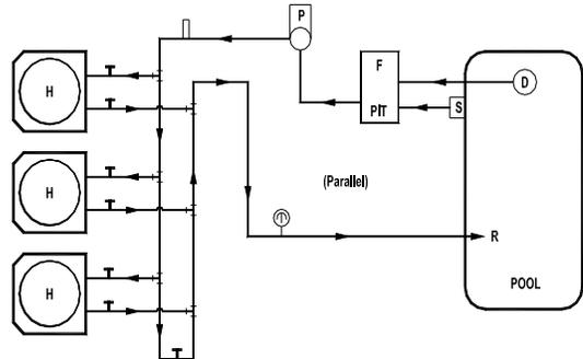
MULTIPLE HEAT PUMP INSTALLATION
