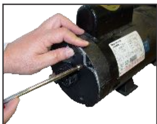
1) Remove the terminal cover off the back off the pump
